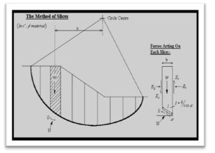
Figure (3) Method of slices: Division of sliding mass into slices and forces acting on a typical slice
