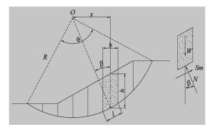
Figure (2) Forces acting on a slice through a sliding mass with a circular slip surface, modified after [9]
