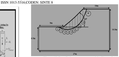
Figure(4) Detail slope geometry with slip surface and location of slices [13]
